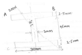
7. Determine the position of the shear center of the section of a beam as shown in fig.
